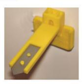
Carefully remove old b lade and place new one in position
