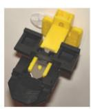
4) Hold the assembly as shown above and slowly fully withdraw the blade carrier ensuring the blade does not fall out.
