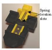
6) Slide the blade carrier with blade back in to the carrier handle approximately half way. Refit the spring in to the slots. Fully slide the blade carrier in until the retaining button clicks in to position.
