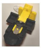
4) Hold the assembly as shown above and slowly fully withdraw the blade carrier ensuring the blade does not fall out.
