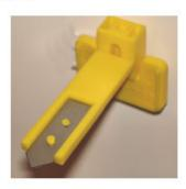
5) Carefully remove old b lade and place new one in position
